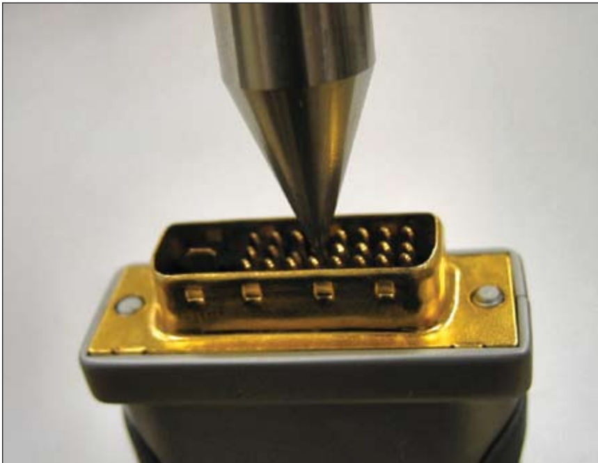
Figure 4: ESD probe easily contacts exposed pins of DVI connector
